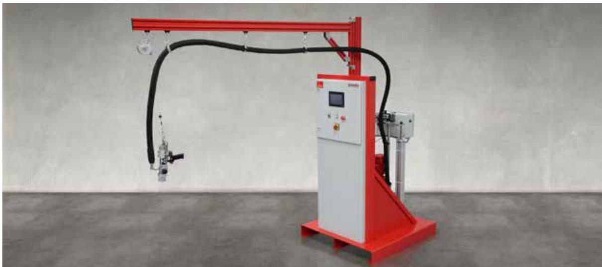
Coredis is used for the processing of especially light low-density 1K epoxies filled with micro hollow spheres. The special challenge in this case is that we are dealing with a reactive medium which remains in the material contacting systems after processing and could be subjected to a curing reaction. In order to prevent this, coredis features a specially developed structure.
