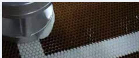
degree of reproducible quality and employee safety. For the first time, the integration into automation solutions allows for a fully automated mass production of honeycomb sandwich panels for aircraft interior equipment.
